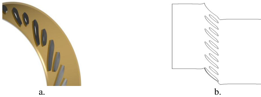
Figure 2-14 Linearization procedure of the annular vaned diffuser configuration a. cylindrical surface at 50% channel height b. unwrapped vaned diffuser (source: Chapter 6 [31])
