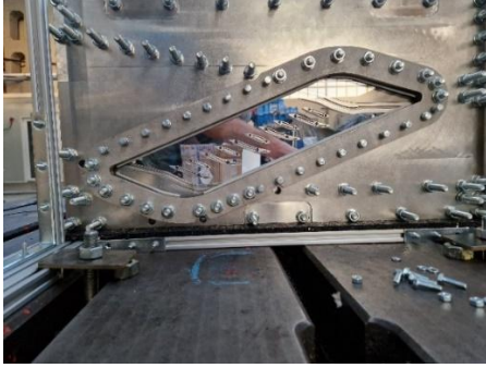
Figure 2-23 Linear cascade side view exploiting optical access (source: Chapter 7 [32])
