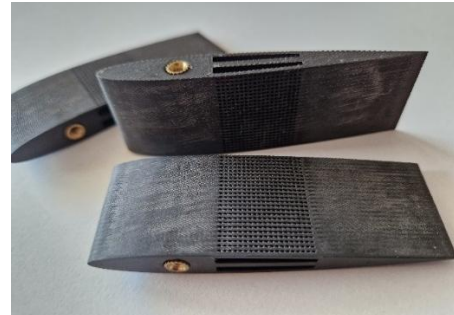
Figure 2-9 Detail of PLA 3D printed airfoil with 0.5 mm hole diameter (source: Chapter 5 [30])
