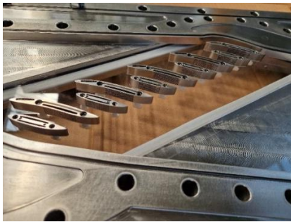
Figure 2-20 Vanes with passive control -front plate quartz optical access window (source: Chapter 7 [32])
