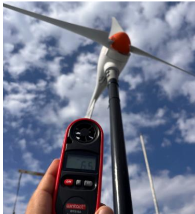
Fig. 0.2. Measuring wind speed at the level of the horizontal axis wind turbine
