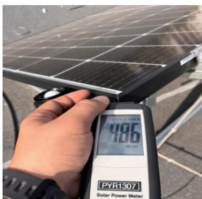
Fig. 0.6. Measuring solar radiation on the inclined surface with the PYR1307 pyranometer
