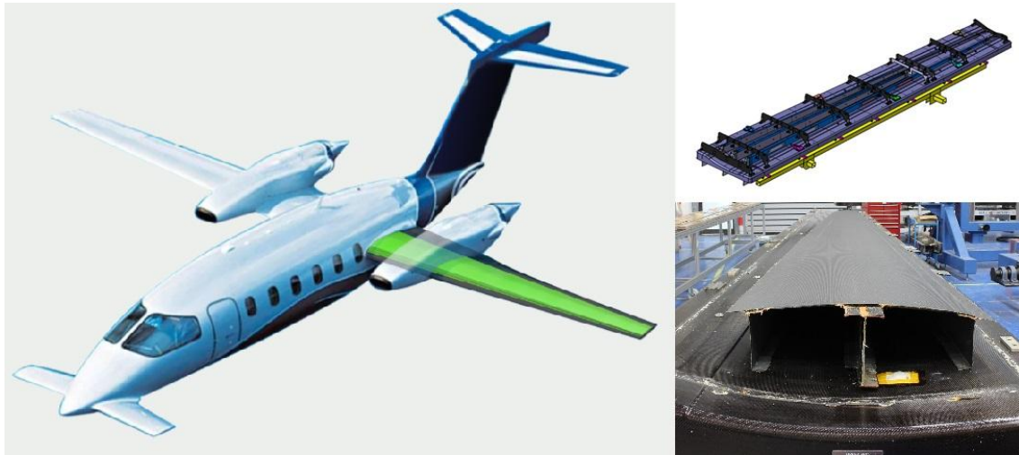
Figure 6.1. The full-scale aeronautical structure simulated for distortion prediction: LEFT - Piaggio P180 aircraft wing, TOP RIGHT - mold for the full skin and spars, BOTTOM RIGHT - 7-meter part fabricated and demolded from the mold.
