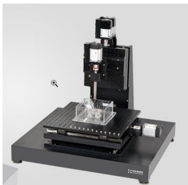
Fig. 1 Holmarc ECDM, model HO-ECDM-0 [5]
