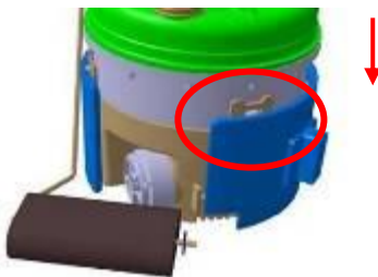
Fig.4.9. Detail of adjacent flexible cylinder embarked on pump mode – fastening and positioning area / anti- rotation
