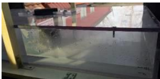
Fig. 7.24. Case S1 with 15L of liquid, without baffle
