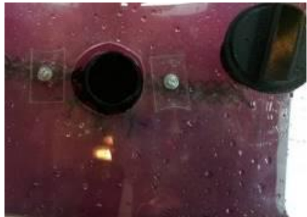
Fig. 7.31. The Fuel delivery module is positioned in the tank while also fixing the wave breaker
