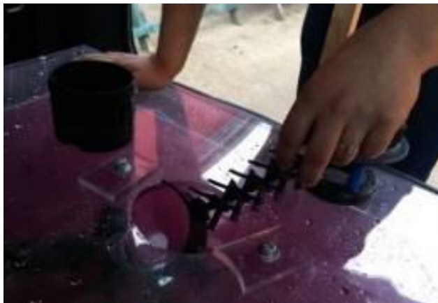
Fig. 7.30. The Fishbone baffle is inserted into the tank through the tank hole intended for the
