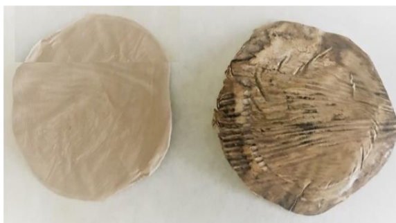
Fig. 9 The appearance of the membrane before the passage of medicines (without magnetite (left) and with magnetite (right))
