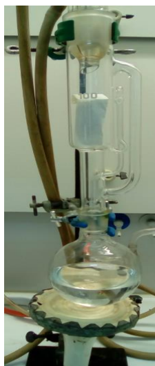
Fig. 4.15. The experimental set-up used for Soxhlet extraction
