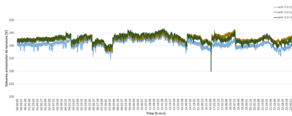
Figure 3.31 The variation of the harmonic voltage gives order 1 on the three phases in April
