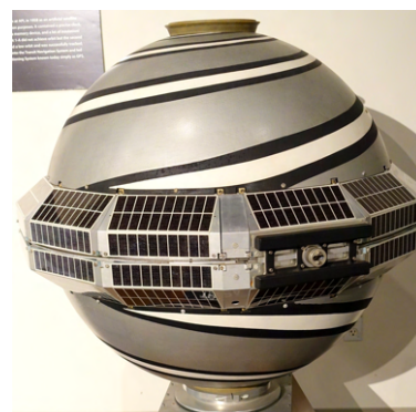
Figure 2.3: Transit-2A navigation satellite model (source: https://commons.wikimedia.org )
