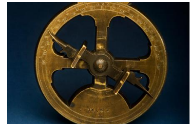
Figure 2.1: A mariner's astrolabe measures the angle of the Sun or a star above the horizontal line of reference (source: https://timeandnavigation.si.edu )
