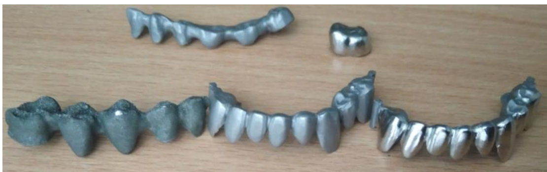
Fig. 8. Dental prostheses realized by selective laser deposition in different states of post-processing
