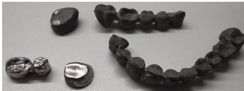
Fig. 3. NiCr dental prostheses made by selective laser deposition in raw/finished state
