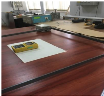
Figure 2.21. The positioning of the calibrated EFA-300 (left) and Extech (right) field-meters for the comparative measurements
