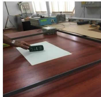
Figure 2.21. The positioning of the calibrated EFA-300 (left) and Extech (right) field-meters for the comparative measurements
