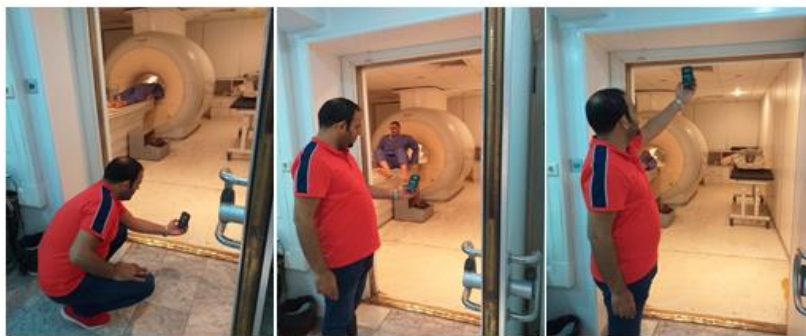
Figure 4.4. The MF measurements at 3 distances (0.3-meter, 1 m and 2 m) from floor.
