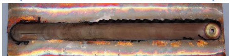
Fig. 7.2.3. Process temperature, axial process force (a) and the aspect of the welded joint (b) at FSW welding - exp. 1.1 (n = 1200 rpm, w = 90 mm/min)
