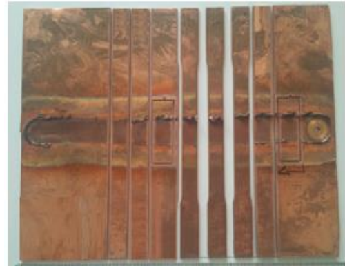
Fig. 7.1.1. Image of a welded structure in the preliminary research (exp. 1.1) and of the specimens sampled from it
