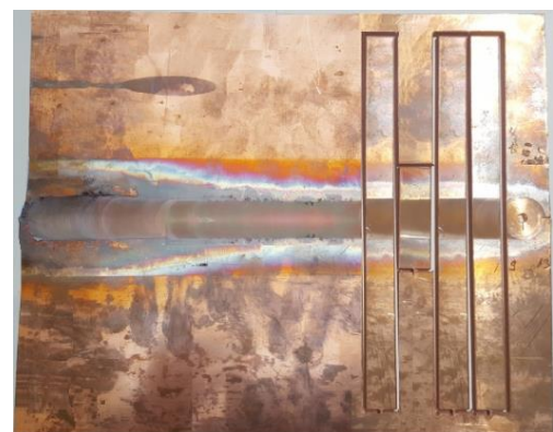
Fig. 8.1.1. Image of a welded structure in advanced research (exp. 2.10) and of the specimens sampled from it
