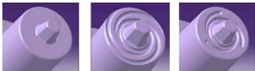
Fig. 1.6.3. Types of channels on the active surface of the active element shoulder [G02]
