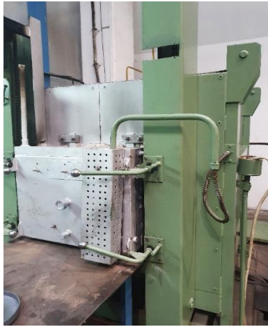
Figure 5.8. Heat treatment furnace used for hardening specimens
