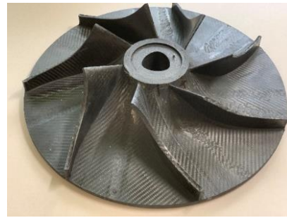
Composite rotor mass – 2,227 Kg
