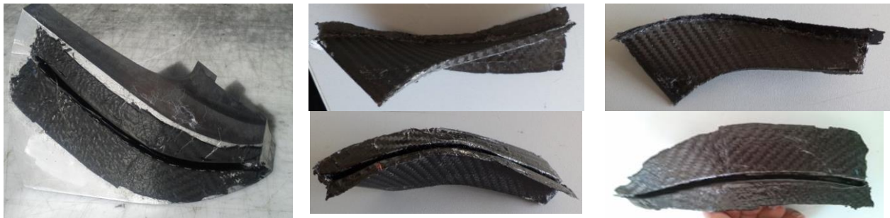
Figure 5.8. Composite rotor blade (1:1 scale) after first technological test
