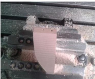
Figure 5.6. Machining and assembling of Necuron moulds
