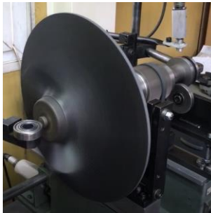
Composite rotor assembly during the balancing process
