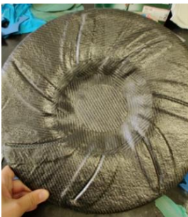
Placing the prepreg layers in the hub area
