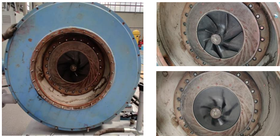
Figure 6.8. Composite centrifugal rotor mounted on the test bench
