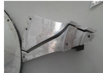
Machined moulds needed for blade manufacturing
