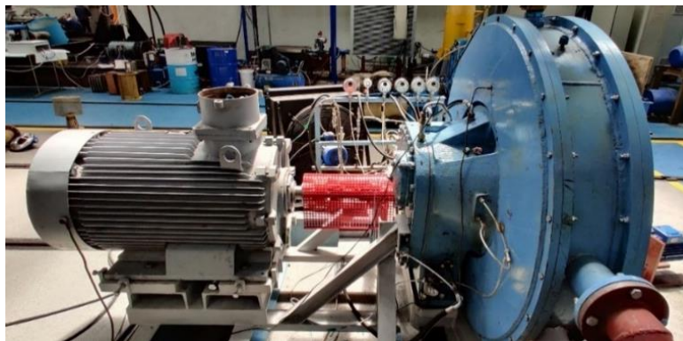
Figure 6.7. Experimental test bench for the validation of the composite rotor
