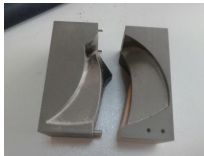
Figure 5.6. Machining and assembling of Necuron moulds
