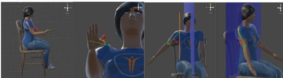
*Fig. 8-2 The angles considered for evaluating the movement score for Forearm Flexion-Extension, Thumb Opposition, Arm Adduction-Abduction, Arm Anteduction-Retroduction*
