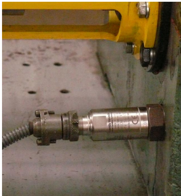
Figure 4.8. Bently Nevada vibration transducer
