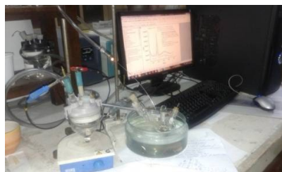
Fig. 6.1. Electrochemical cells used in electrochemical and metal detection
