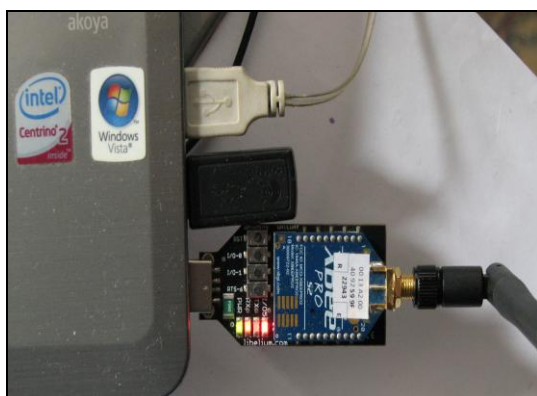
Figure7.5 Nodul Coordonator conectat la laptop
